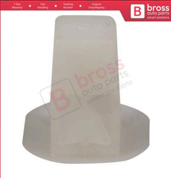
BCF1843 10 Pieces Screw Grommet for Nissan Head Diameter 15.3mm Fits into hole 8mm
